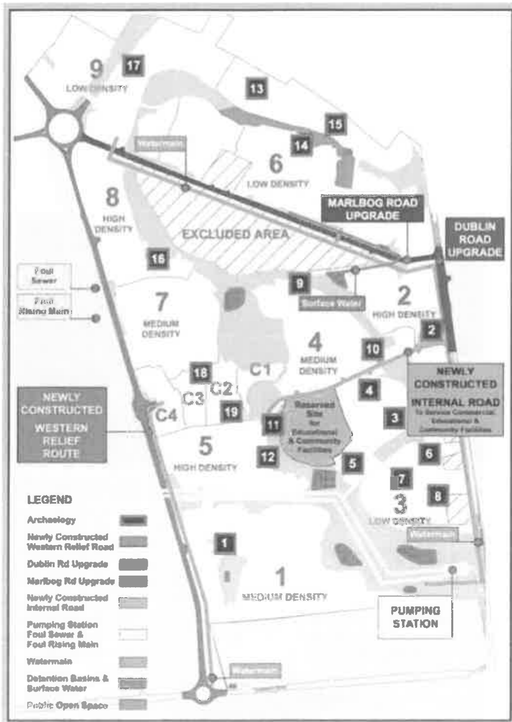
Figure 3. Overview of Infrastructure and Enabling Works undertaken at Haynestown Development Site
